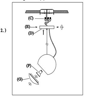
Step.2: Adjust wire length to desired mounting height, and tighten strain relief screws to secure. Wire fixture to wires in outlet box. Green wire is for Ground. Install fixture to bracket and tighten screws (E) at the ends of the canopy (D) to secure. Install LED GU10 bulb (F) and attach diffuser (G) to concrete shade. Direct shade using spring coil cable.
