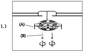
Step.1: 1: Remove mounting bracket (A) from fixture and install to electrical box using screws (B).
